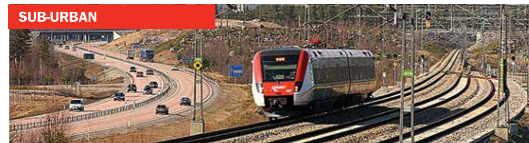
Commuter rail, also called suburban rail, is a passenger rail transport service that primarily operates between a city center and the middle to outer suburbs beyond 15 km.
